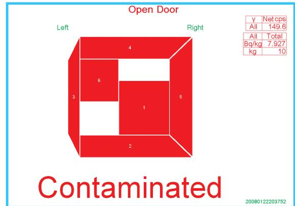
This display will show the quantity and location of the contamination based on which of the detectors is alarming, unless alarm is set on sum zone only. The operator opens the door, removes the object(s) and closes the door. The Cronos-1 will then perform a detector contamination check automatically to ensure there is no detectable amount of radioactivity remaining in the unit.
