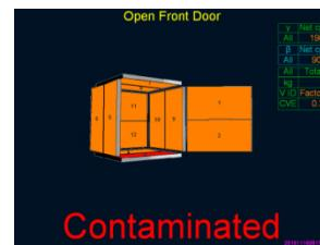
This display will show the measured count rate and the location of the contamination based on which of the 12 detectors is/are alarming. The operator opens the door, removes the object(s) and closes the door.
